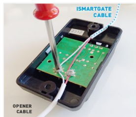
Wire the ismartgate outputs to the screws on your push button. Polarity does NOT matter. Then screw again.
