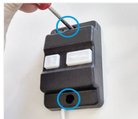
Unscrew the push button from the wall.
